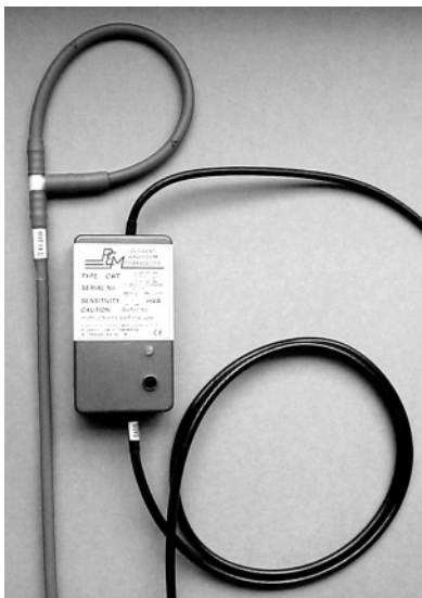
Fig. 1. Rogowski transducer showing flexible coil, electronic integrator and interconnecting cable.
