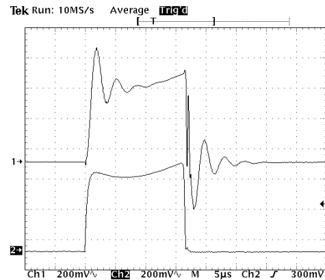
Fig. 13. Measurement of current pulse (200A/div) UPPER: LEM-flex; LOWER CWT30
